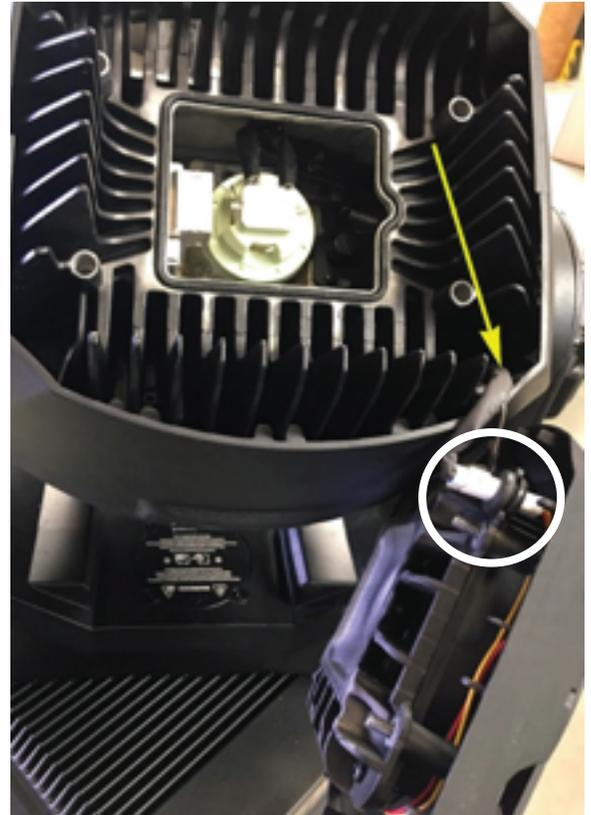
2. Unscrew the (4x) allen head screws to remove the rear cover. When removing the rear cover, please be advised that the cover is connected to the unit via a safety cable and connected wire cable.
