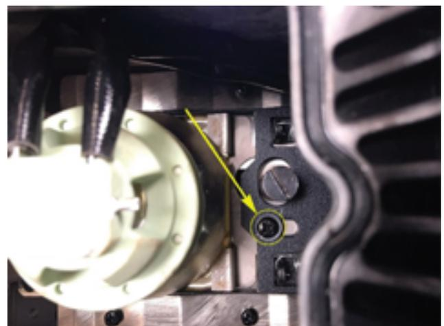
4. Loosen the Phillips head screw to unlock the lamp holding slider.
